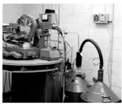
Freezing apparatus in the Rossmann lab for collecting the first data from frozen LDH crystals.
