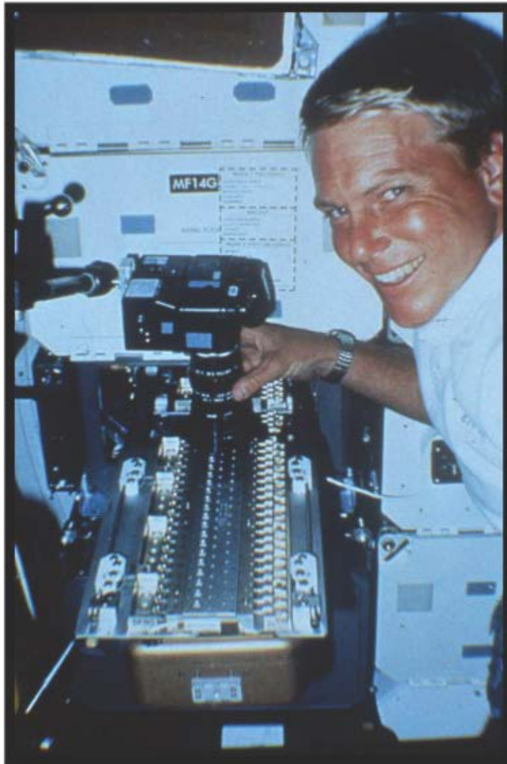
Figure 20: Payload specialist Pinky Nelson (no kin to Congressman Nelson) training with the Advanced VDA, which was constructed following the Challenger accident. This system was more automated, and the vapor diffusion apparatus was housed in a special temperature controlled unit that was designed to replace one of the mid-deck lockers on the Space Shuttle. Pinky performed our first experiments with the Advanced VDA on Space Shuttle Flight STS-26, which launched on September 29, 1988.
