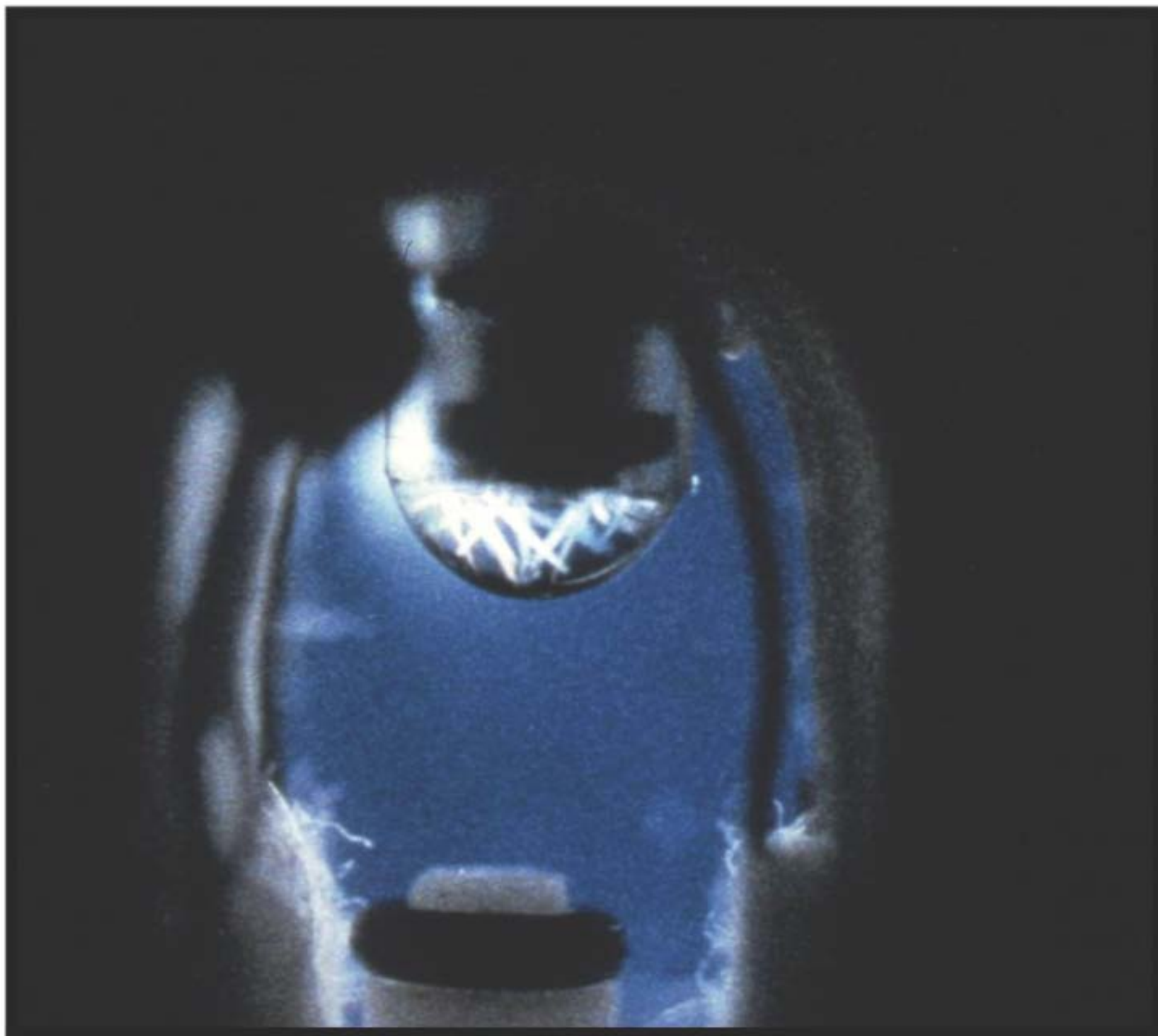
Figure 13: Details of a single crystal growth chamber in the VDA. The plunger that seals the protein syringe during launch and landing is shown in the retracted position at the bottom of the chamber. The extruded protein solution is shown on the tip of the syringe at the top, with protein crystals growing within the droplet.
