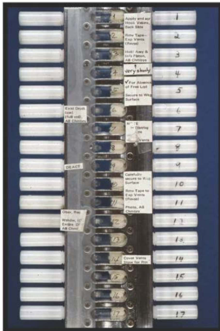
Figure 12: The Handheld Vapor Diffusion Apparatus (Handheld VDA) flown on Space Shuttle Flight STS-51D. The apparatus contains seventeen chambers, each with a separate protein crystal growth experiment. Each chamber contains an absorbent wicking material, shown at the right of the chamber, which was saturated with the solution of precipitating agent prior to launch. The white cylinders protruding from the sides of the chambers are syringes, which are operated by an allen wrench. The syringes containing protein solutions are shown at the left of the chambers. The syringes on the right operate plungers that seal the tips of the protein syringes during launch and landing. The syringes on the left extrude droplets of protein solution, which then equilibrate with the precipitating agent within the chamber. Prior to landing, the protein droplets are withdrawn into the syringes and the syringes are sealed. Notes are shown attached to the apparatus as reminders of the steps for Charlie Walker to follow.
